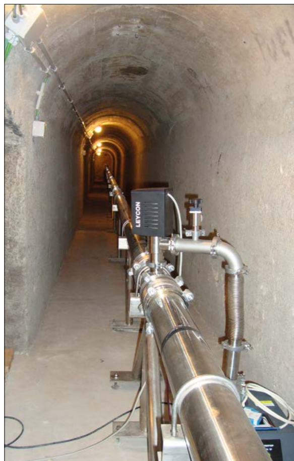
One section of the 70 m laser strainmeter installed at the LSC to study local and global geodynamic events.
