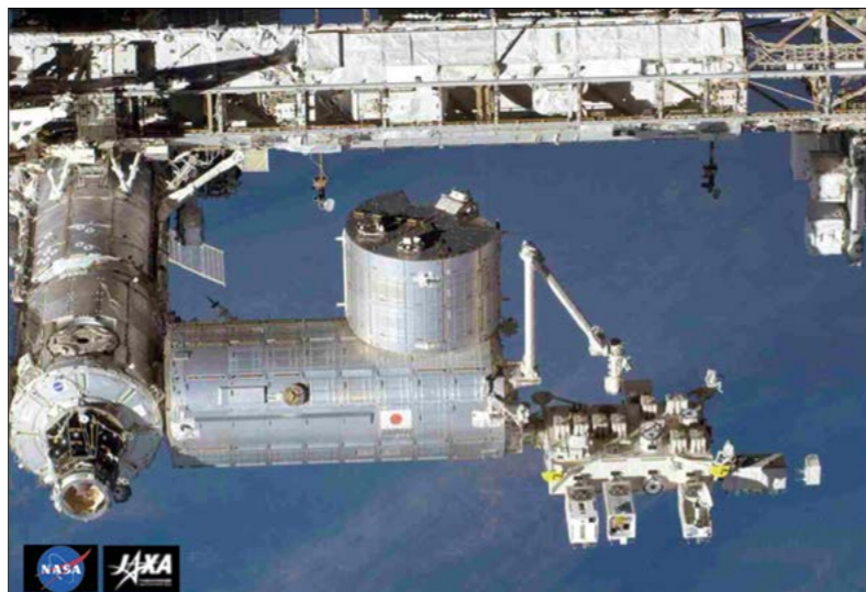
After berthing with the ISS, CALET was extracted by robotic arm from the Japanese HTV-5 transfer vehicle and installed on the Japanese Exposure Facility (right), where it will start its first data-taking. (Image credit: NASA, JAXA.)
