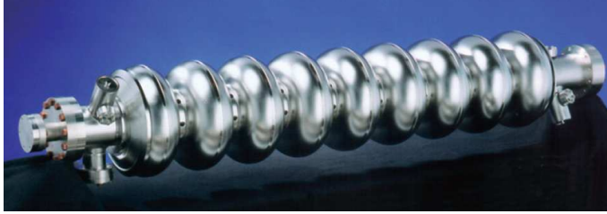
Figure 1: A superconducting niobium cavity designed for a high-energy e^+e^- linear collider. The cavities operate at radio frequencies and can support fields up to 50 \text{ MV m}^{-1} .
