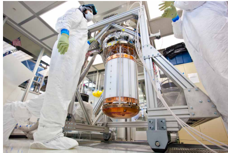
Figure 8: Dark matter detectors require low radioactive backgrounds, and are operated deep underground to shield them from cosmic rays. Some make use of copper from sunken Roman ships, which has particularly low induced radioactivity because it has been shielded from cosmic rays by the sea for centuries.
