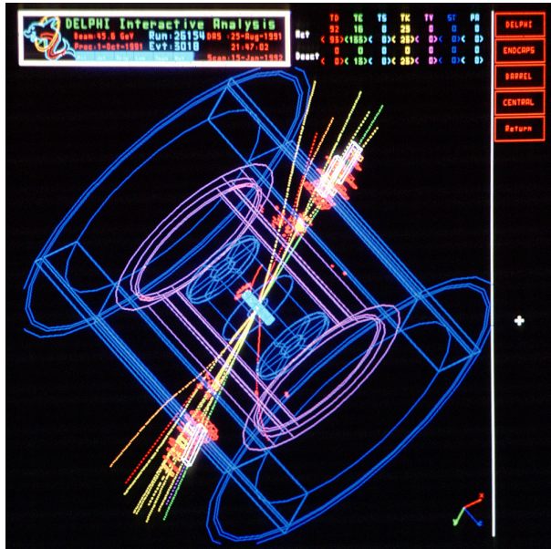
Figure 1: A two-jet event in the Delphi detector at a electron-positron centre-of-mass energy close to 100 GeV. © CERN 1992.
