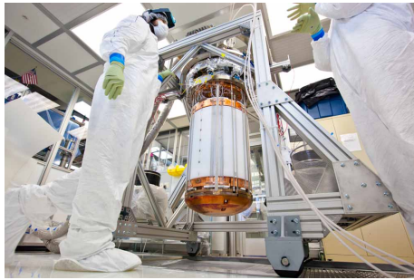
Figure 6.8: Dark matter detectors require low radioactive backgrounds, and are operated deep underground to shield them from cosmic rays. Some make use of copper from sunken Roman ships, which has particularly low induced radioactivity because it has been shielded from cosmic rays by the sea for centuries.
