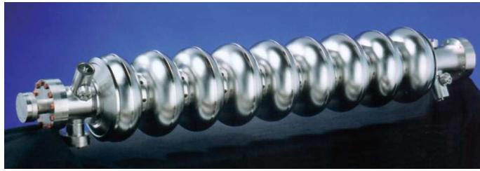
Figure 8.1: A superconducting niobium cavity designed for a high-energy e^+e^- linear collider. The cavities operate at radio frequencies and can support fields up to 50 \text{ MV m}^{-1} .
