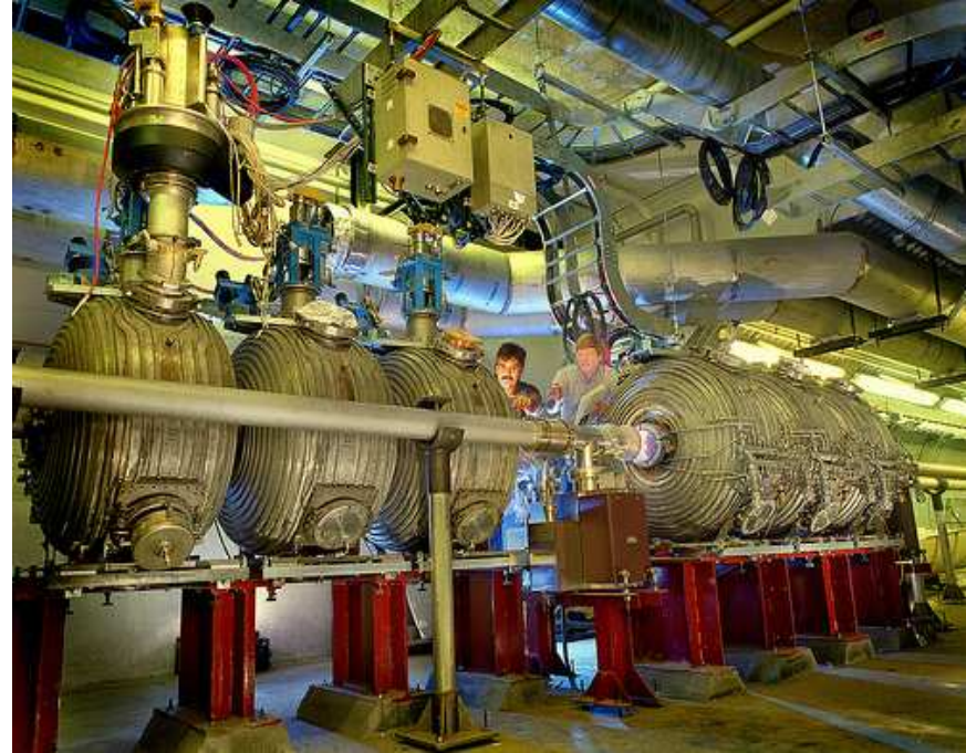
RF-Cavity for RHIC (Relativistic Heavy Ion Collider at Brookhaven National Laboratory)
