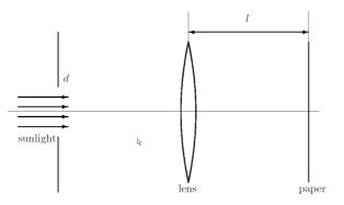
Explain why the light from the sun may be assumed to be collimated. The light intensity coming from the sun is  $S=1.37 {\rm kW/m^2}$ . Calculate the light intensity I arriving at the sheet of paper and the illuminated area A as a function of the distance l.
