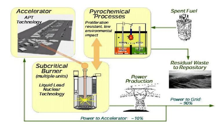
A linac scheme for driving a reactor. These devices can turn thorium into a reactor fuel, power a reactor safely, and burn up long-lived fission products.
