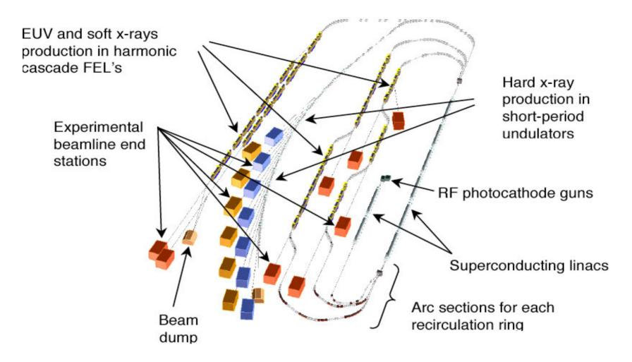
A possible fourth generation light source. This is the proposed facility LUX, as envisioned by a team at LBL. Features a recirculating linac and energy recovery . X-tax pulses of femtosecond length.
