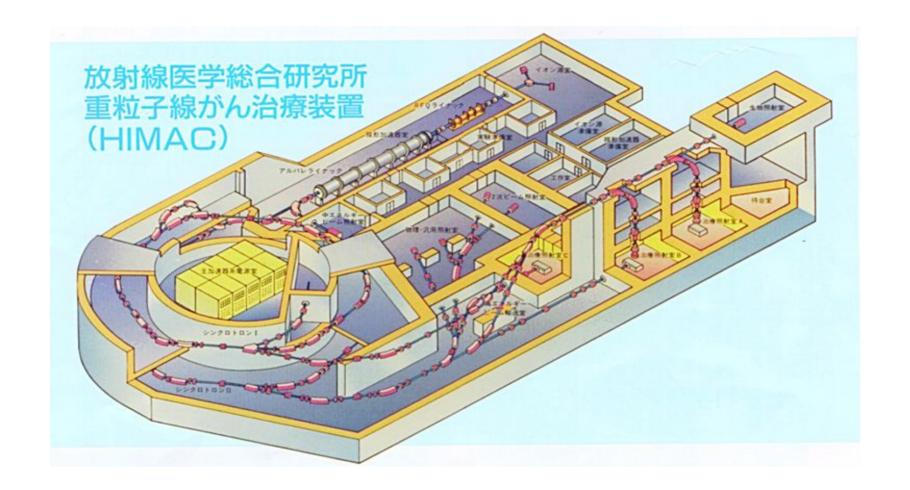
A drawing showing the Japanese proton ion synchrotron, HIMAC. The facility consists of two synchrotrons, so as to maintain a continuous supply of ions (or protons) to the treatment area. The pulse of ions is synchronized with the respiration of the patient so as minimize the effect of organ movement.
