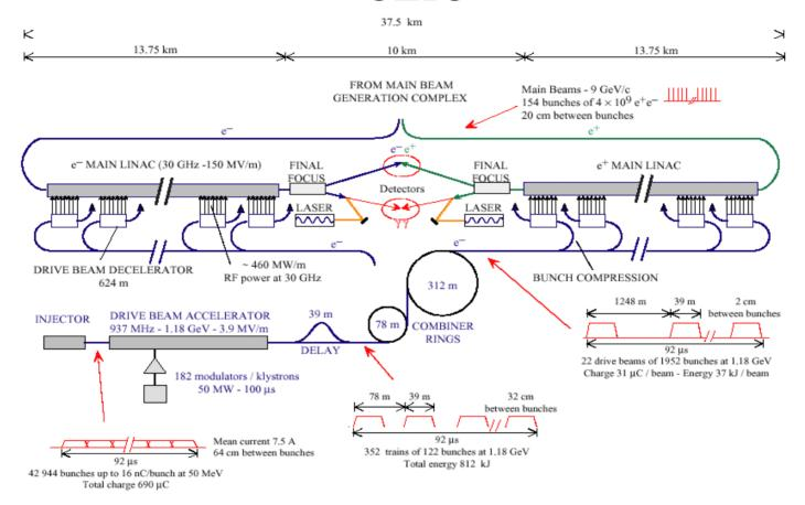
A diagram showing the CERN approach to a linear collider. The two main linacs are driven by 12 GHz radio frequency power derived from a drive beam of low energy but high intensity that will be prepared in a series of rings combined with a conventional linac.
