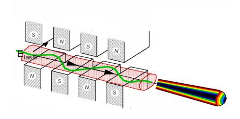
FELs, invented in the late 1970's at Stanford are now becoming the basis of major facilities in the USA (SLAC) and Europe (DESY). They promise intense coherent radiation. The present projects expect to reach radiation of 1 Angstrom (0.1 nano-meters, 10kilo-volt radiation)
