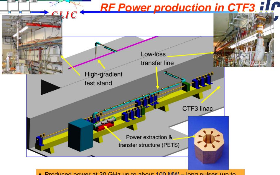
Produced power at 30 GHz up to about 100 MW – long pulses (up to 300 ns) available for the first time
