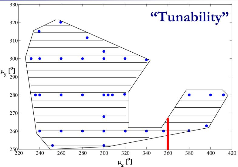
■ Phase advance tunable between 240° and 420° in the horizontal and between 250° and 320° in the vertical plane
