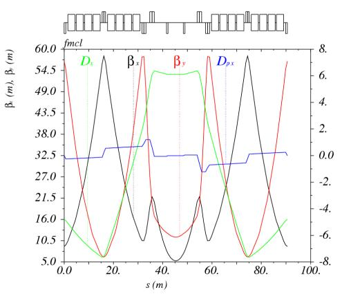
Main disadvantage the length of the module, giving an arc of around 560m (5 modules + dispersion suppressors), versus 510m for the FODO cell arc
