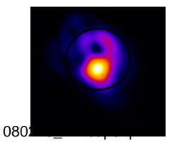
Incident power 24TW, (37 fs, 0.9J) Intensity 9 10<sup>17</sup>W cm<sup>-2</sup> vaccuum Capillary output
