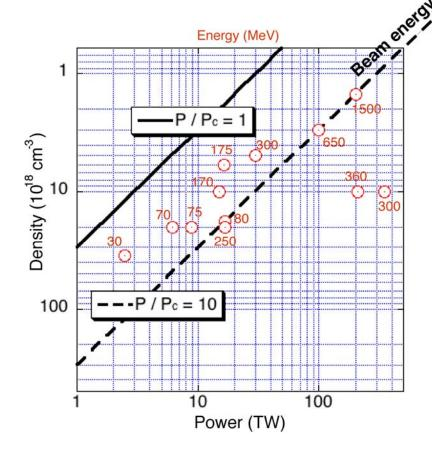
The increase of laser power allows to decrease electron density and maintain self-focusing (to compensate diffraction)
