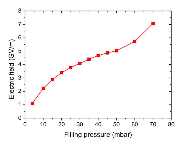
Electric field of the plasma wave deduced from optical diagnostic
