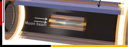
Detector comprised of pixel tracker + scintillating fibres
