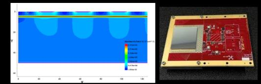
The project will focus on developing operational pixel LGADs, by simulating them, developing calibration algorithms, and testing their performance in the lab and at beam facilities
