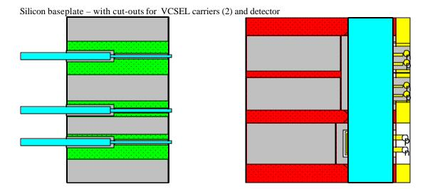
Silicon lid (with v-grooves and fibres) and baseplate / tile / mirror assembly
